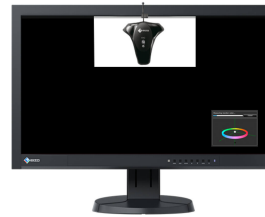
Recording white point and brightness values when calibrating with an external sensor
